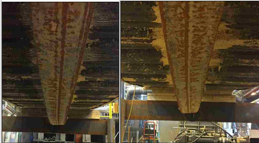
Figure 54 – Test 3 Beam Twist at Failure
