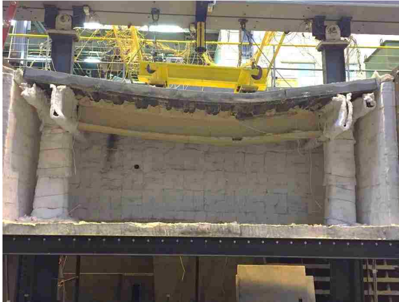
Figure 50 – Protected Beam after Failure
