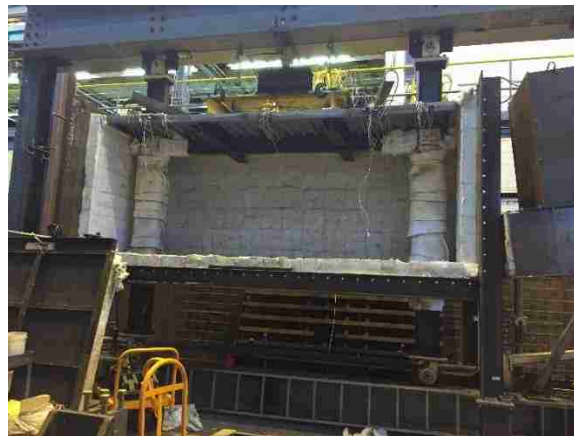
Figure 6 – Protective Ceramic Blankets on Columns and Beam Connections
