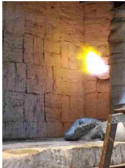
Figure 4 – Maxon Kinemax 3” Series G Burner while Ignited.
